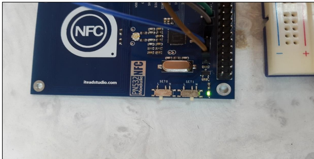
Fig. (3.3): The Setting of SET0, SET1 Switches of NFC Module
