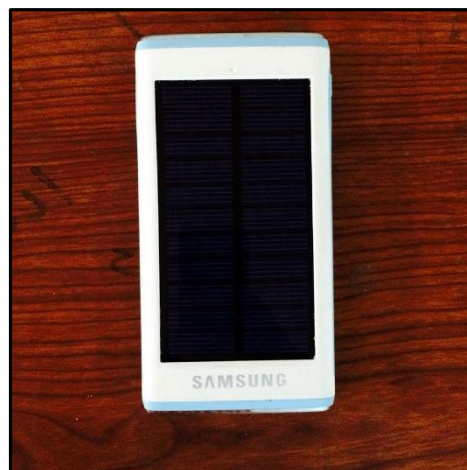
Fig. (2.8): The Solar Cell Used as a Power Supply in This Project.
